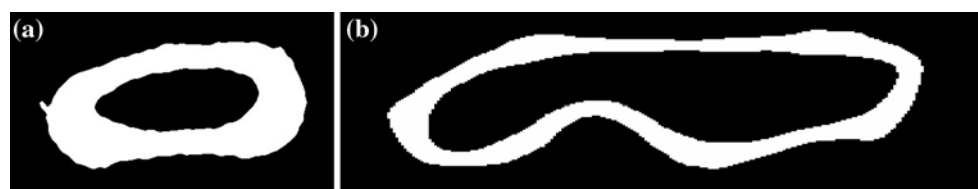
Fig. 11 Cross sections of dried (a) latewood kraft pulp fibre and (b) earlywood kraft pulp fibre
